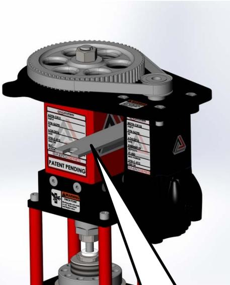
WITH SPACER TOOL IN PLACE, TIGHTEN CAP SCREWS TO 79 IN\* LBS AND REMOVE SPACER
