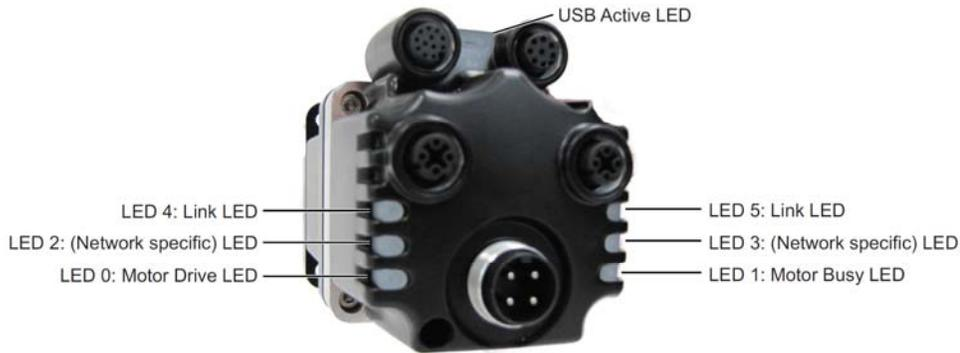
Flickering = On/Off in 0.1 sec; Blinking = On/Off in 0.5 sec; Flashing = separated by 1 sec for EtherCAT LEDs and 2 sec for Fault Codes
