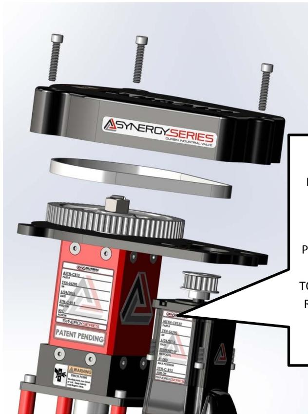
HAND TIGHTEN ALL (4) MOTOR MOUNTING SCREWS AND SLIDE MOTOR TOWARDS ACTUATOR TUBE.
